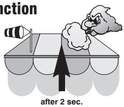
As long as the measured wind speed is higher than the adjusted threshold, all commands are prevented from operating. (manual control or automatic control).
