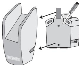
2. Loosen the strain relief plate and guide the power supply wires through the black grommet into terminal block.
