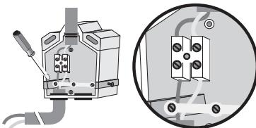
3. Connect the cable leads to the terminals
