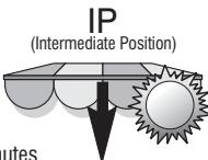
When the daylight level falls below the threshold setting, a variable time delay from 15 to 30 minutes is activated (depending on the sun presence duration). *This feature avoids frequent movements of the awning on cloudy days.*
