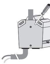
5. Attach the sensor to the wall.
